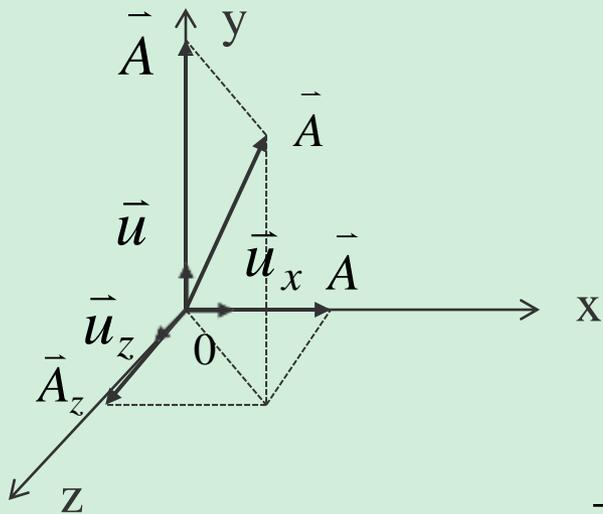
$$\begin{aligned} \vec{A} &= \vec{A}_x + \vec{A}_y + \vec{A}_z \\ &= A_x \vec{u}_x + A_y \vec{u}_y + A_z \vec{u}_z \end{aligned}$$
