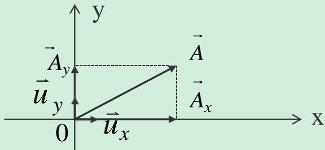
$$\begin{aligned}\vec{A} &= \vec{A}_x + \vec{A}_y \\ &= A_x \vec{u}_x + A_y \vec{u}_y\end{aligned}$$
