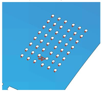
4. Show the entire model. Select **Solid > Remove and Extend** and select all the holes (by box) **except for the hole indicated by the arrow in the picture below**.
