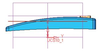
5. Create a **New Extrude** operation. Select the previously created curve as the input curve.
