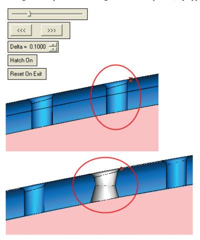
4. Create intersection curves between the inner faces of the hole and the datum plane as shown in the pictures below.
