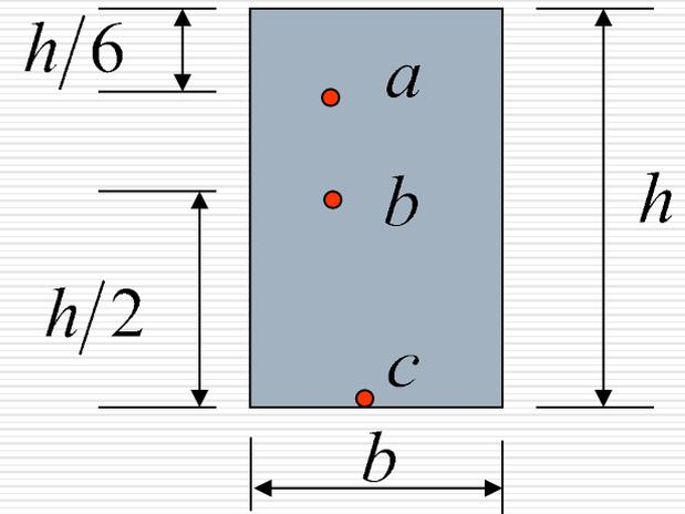
$$\sigma_a = \frac{M_B y_a}{I_z} = \frac{\frac{1}{2} FL \frac{h}{3}}{\frac{bh^3}{12}} = 1.65 \text{ MPa}$$
