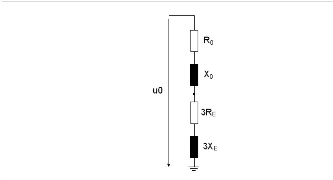
Figure 5.2: NEC - Equivalent circuit in the zero system
