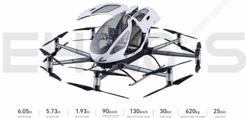
EH216-S: Pilotless Passenger-Carrying eVTOL for Intra-City Air Mobility
