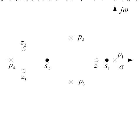
(1) 在  $[z_1 \ p_1]$  区间上取一点  $s_1$  ,由各开环零极点向该点分别引矢量,如图所示。设  $\angle(s_1-z_j) = \varphi_{1j}$  ,则有: $\angle(s_1-p_i) = \theta_{1i}$   $\theta_{12} = -\theta_{13}$   $\varphi_{12} = -\varphi_{13}$
