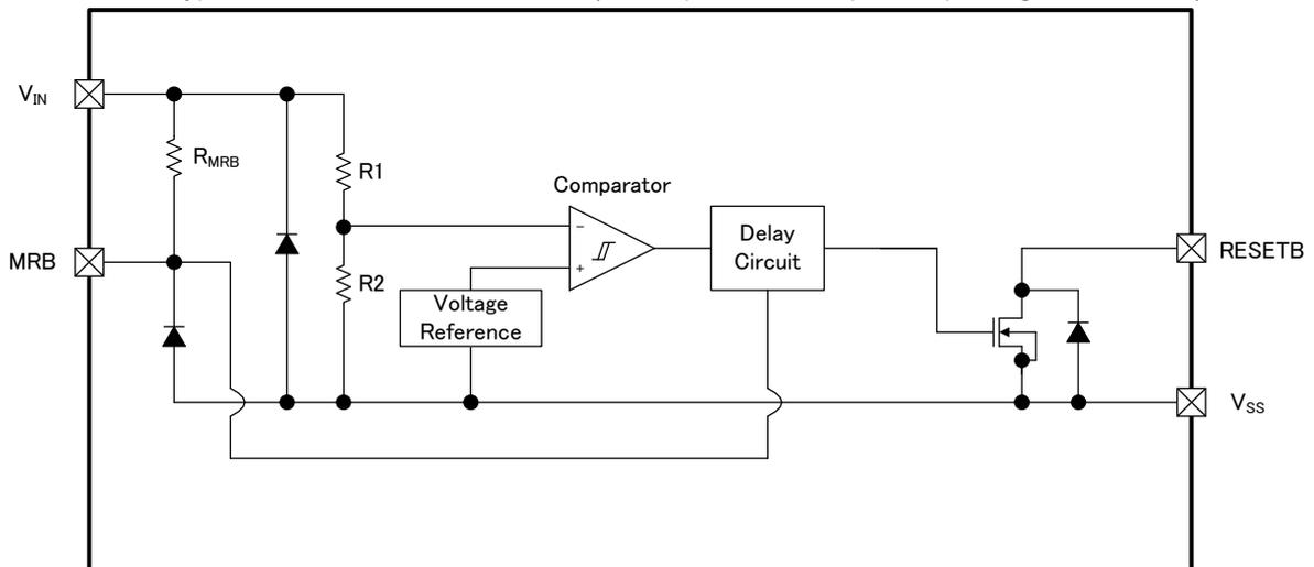
\* Diodes inside the circuits are ESD protection diodes
