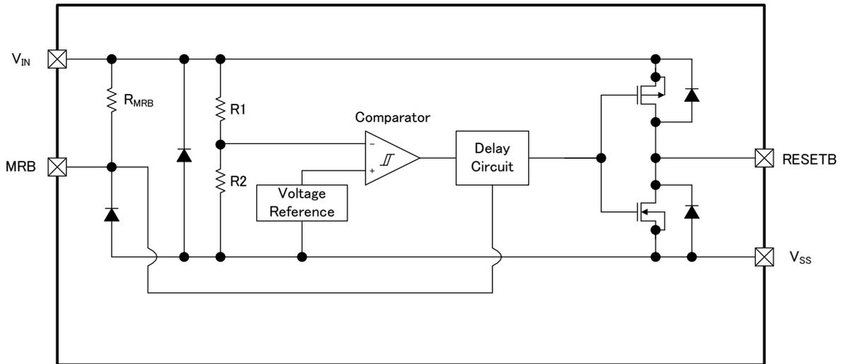
\* Diodes inside the circuits are ESD protection diodes and parasitic diodes.
