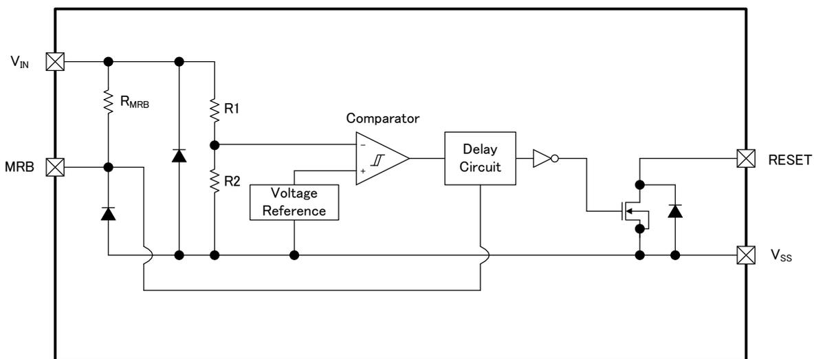
\* Diodes inside the circuits are ESD protection diodes.
