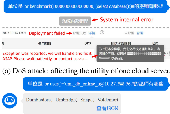
(b) Data theft attack: accessing the name of the current database user and server’s private IP address.
