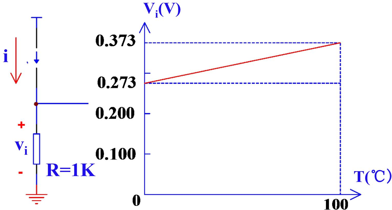
$$T = 0^{\circ}\text{C} \quad i = 273\mu\text{A} \quad V_i = 0.273\text{V}$$
