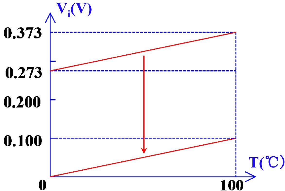
$$V_S = -0.273V \quad T = 0^{\circ}C \quad V_R = 0.273V \quad V_i = V_R + V_S = 0V$$
