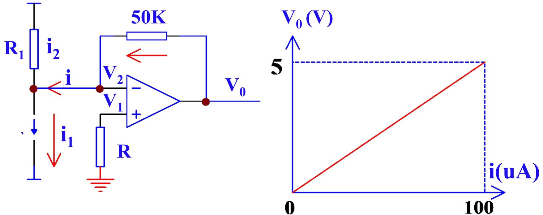
$$V_1 = V_2 = 0$$
