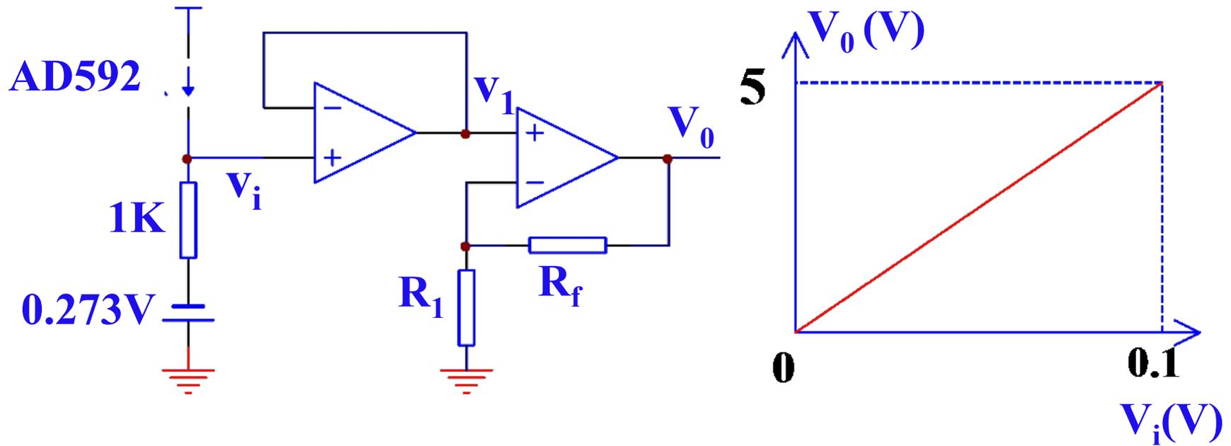
$$V_1 = V_i, \quad V_0 = V_1(1 + R_f/R_1)$$
