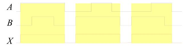
The OR operation can be used in computer programming to set certain bits of a binary number to 1.
