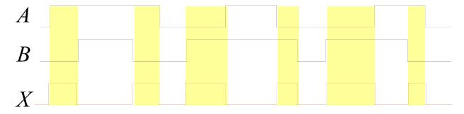
Notice that the XOR gate will produce a HIGH only when exactly one input is HIGH.
