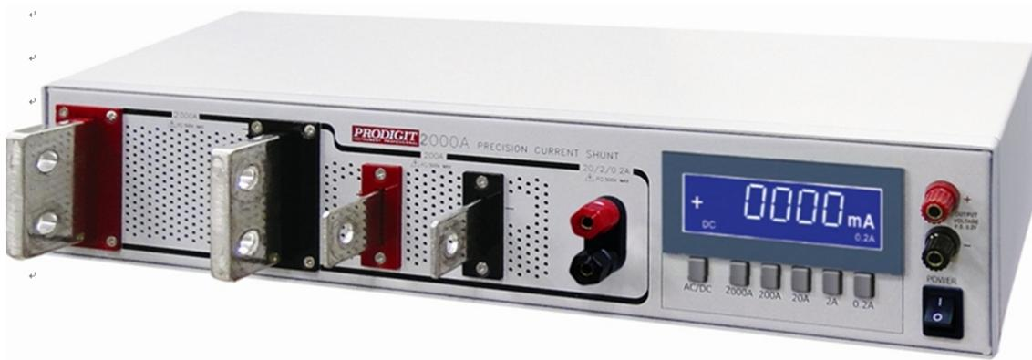
The compliance voltage of the shunt is less than 0.2 volts at full scale for each range except the 2000 Ampere range which has a compliance voltage of 0.02 volts. The shunt is a highly stable AC/DC resistor connected in a four-terminal non-inductive configuration for each range.
