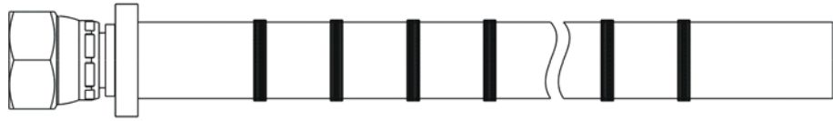
Fig. 4-9: Water line, green
