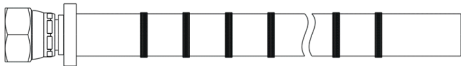
Fig. 4-10: Water line, green
